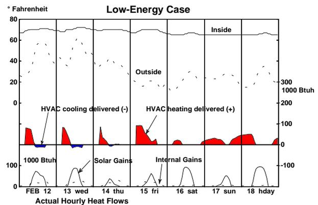
Figure 5. Hourly simulation results for 7 days in February. HVAC graphs show energy delivered to the building (+) or removed from the building (-) by the HVAC system. Another plot (not shown) indicates energy into the HVAC system.
