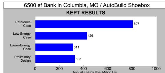
Figure 6. An example of a KEEP graph. Results “kept” for each of the four cases shown can be displayed. The example displays annual energy use, however, there are 10 other plotting options (heating, cooling, cost, peak electric use, etc.).
