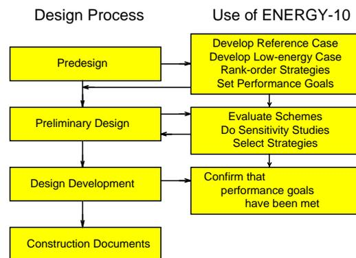
Figure 1. How *ENERGY-10* integrates into the design process.
