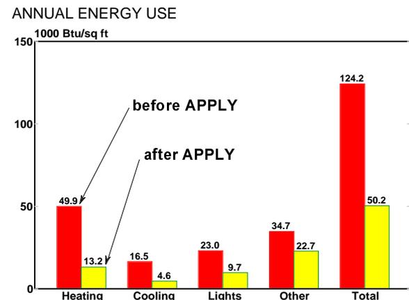
Figure 2. Building performance before and after 10 energy-efficient strategies are applied in combination
