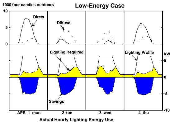
Figure 7. Results of the dimming of lights resulting from available daylight in the building for 4 days in April. The lighting profile is the total required light, the savings (shown inverted for clarity) is the amount of dimming, and the lighting required is the difference between the two.
