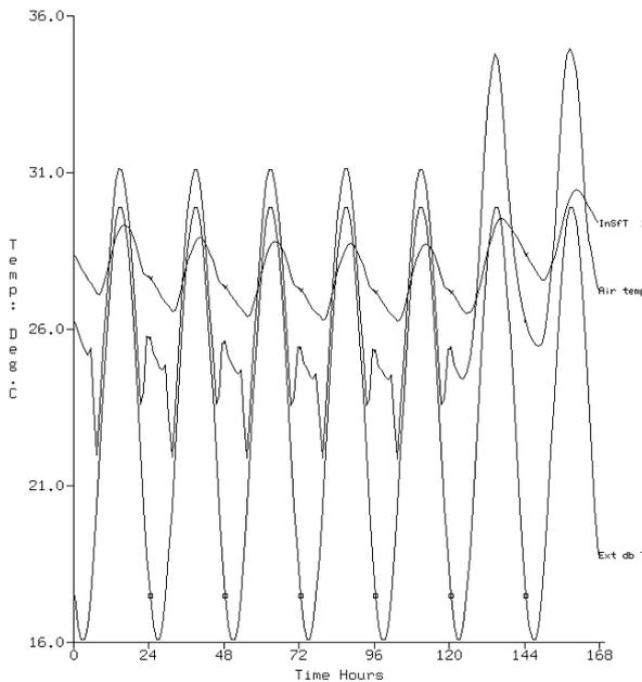
**Figure 5** : Internal air temperature  $t_i$  and floor surface temperature  $t_s$  as a function of external and internal conditions during the working week and weekend (external air temperature  $t_e$ )
