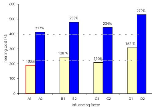
**Figure 1:** Variation of costs and energy consumption for heating of the flat during one-week depending on flat location, increased set-point, neighbouring apartment and excessive ventilation (price is 163KC per GJ)
