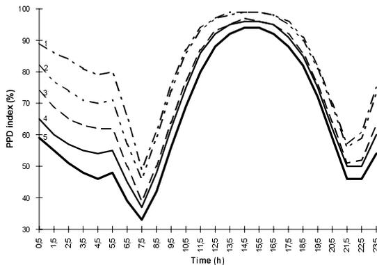
**Figure 7 :** Thermal discomfort - PPD index - as a function of skylight area and floor construction during the working day: 1-Skylights 6 x 5 m, floor light, ther. insulated, 2-Skylights 6 x 5 m, floor heavy, ther. non-insulated, 3-Skylights 6 x 3 m, floor light, ther. insulated, 4-Skylights 6 x 3 m, floor heavy, ther. insulated, 5-Skylights 6 x 2 m, floor light, ther. Insulated
