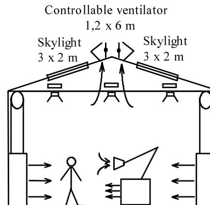
**Figure 4:** The displacement ventilation system and its operation during the summer period in an industrial hall
