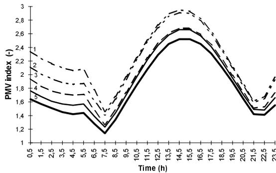
**Figure 6 :** Thermal comfort sensation - PMV index - as a function of skylight area and floor construction during the working day, 1-Skylights 6 x 5 m, floor light, ther. insulated, 2-Skylights 6 x 5 m, floor heavy, ther. non-insulated, 3-Skylights 6 x 3 m, floor light, ther. insulated, 4-Skylights 6 x 3 m, floor heavy, ther. insulated, 5-Skylights 6 x 2 m, floor light, ther. insulated
