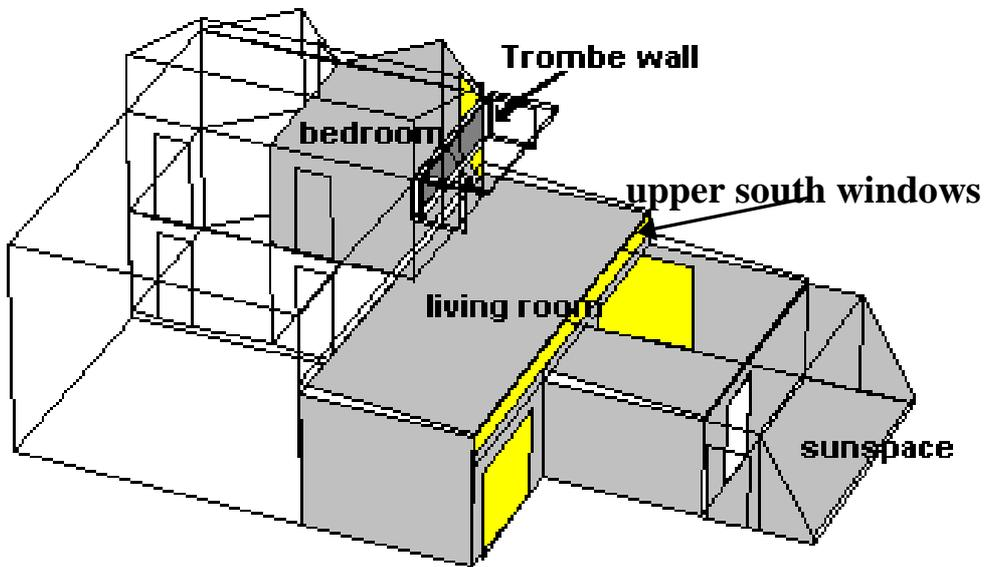
Fig. 2: Global model with eleven thermal zones.
