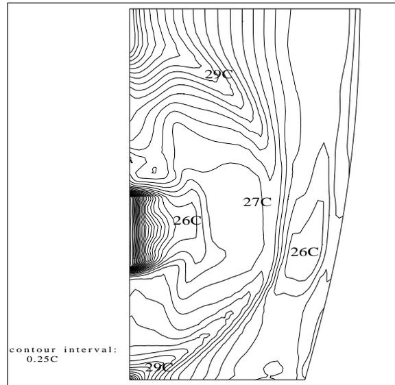
**Figure 11.** Horizontal temperature distribution under full load conditions, mechanical supply  $21^\circ\text{C}$  at about  $1\text{m}^3/\text{s}$
