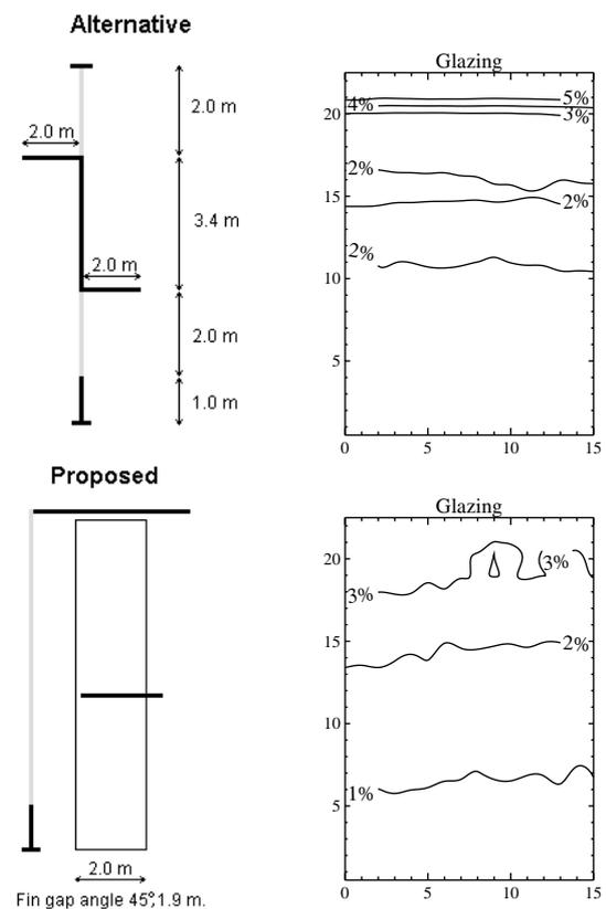
**Figure 8 Alternative and proposed facade glazing and shading with predicted daylight factors across a section of the banquet hall**
