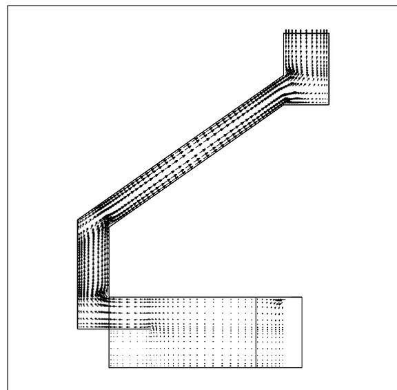
**Figure 12.** Air flow in banqueting hall under night time venting conditions, intake open area  $25\text{m}^2$ , surface temperatures  $26^\circ\text{C}$ , ambient temperature  $20^\circ\text{C}$  (a vector of  $1\text{cm}$  corresponds to a speed of  $4\text{m/s}$ )
