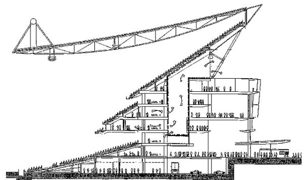
**Figure 5 Section through stadium showing banquet hall and vent shaft**
