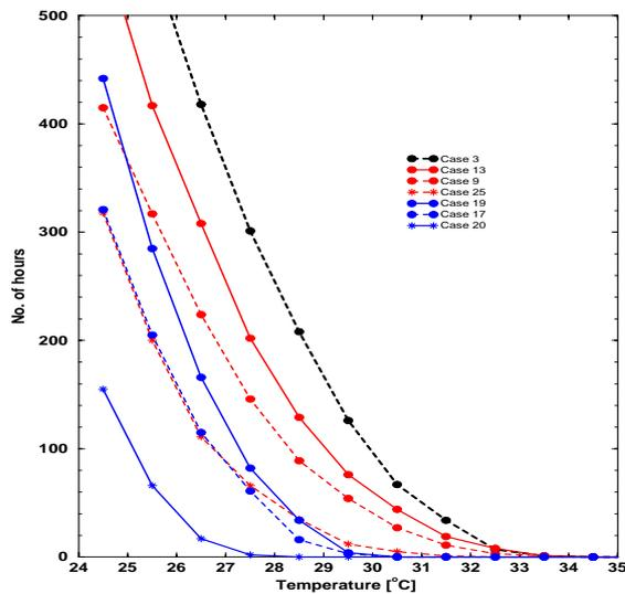
**Figure 10** Cumulative number of hours for which particular dry resultant temperatures are exceeded in naturally controlled option
