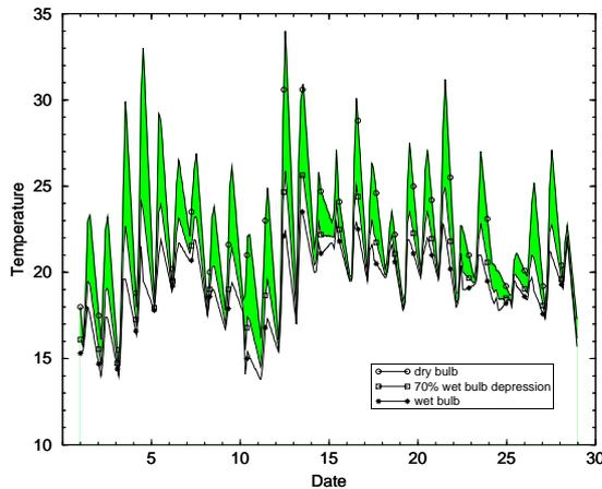
**Figure 4 Hourly dry bulb and wet bulb temperatures in February and theoretical temperature reduction by evaporative cooling**
