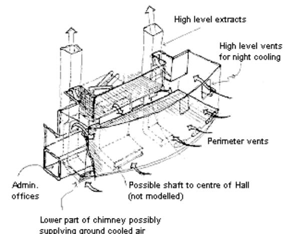
**Figure 6 Axonometric of initial ventilation strategy proposed for the banquet hall**
