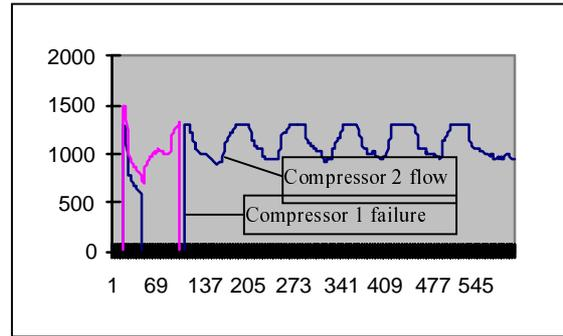
Figure 4: Flow Response to Compressor 1 Failure
