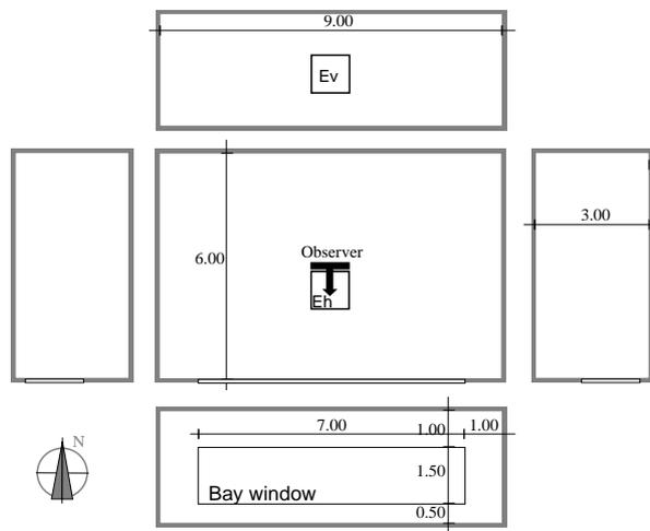
Fig. 3: Test cell plan
