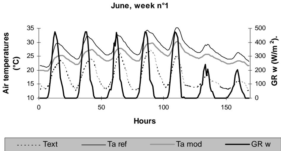
Fig. 9: Effect of the modification of the transparency of the window (from visual comfort criteria) on the indoor air temperature. GR w is the vertical global radiation on the window.
