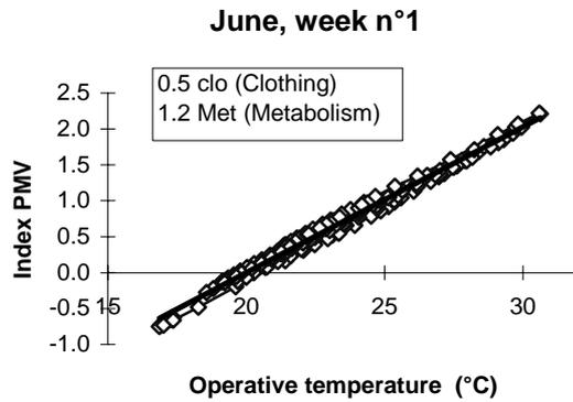
Fig. 11: Evaluation of PMV from operative temperature
