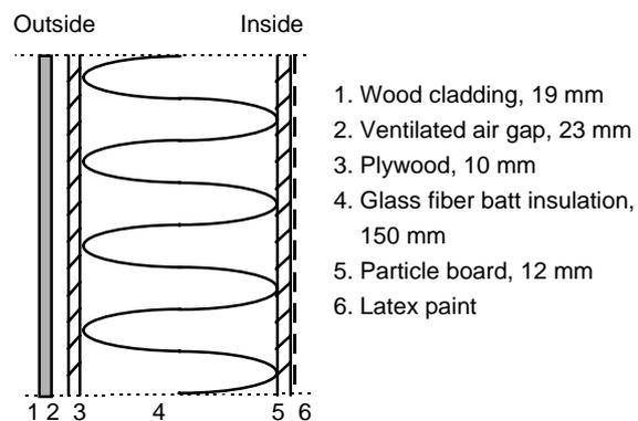
*Figure 1 The constructional design of the wall*
