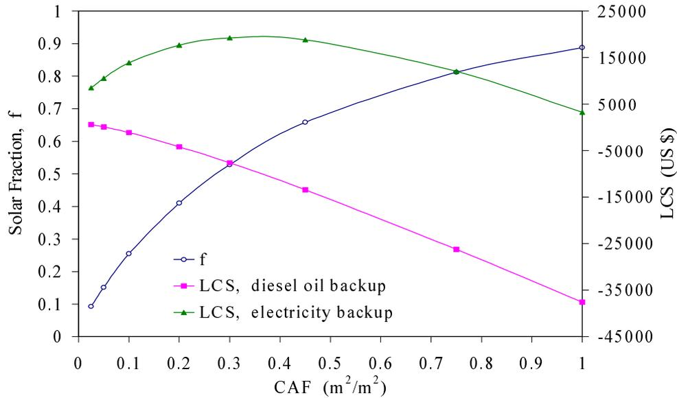
Fig. 2. Annual solar fraction and life cycle savings as a function of the collector to building floor area criterion (CAF).
