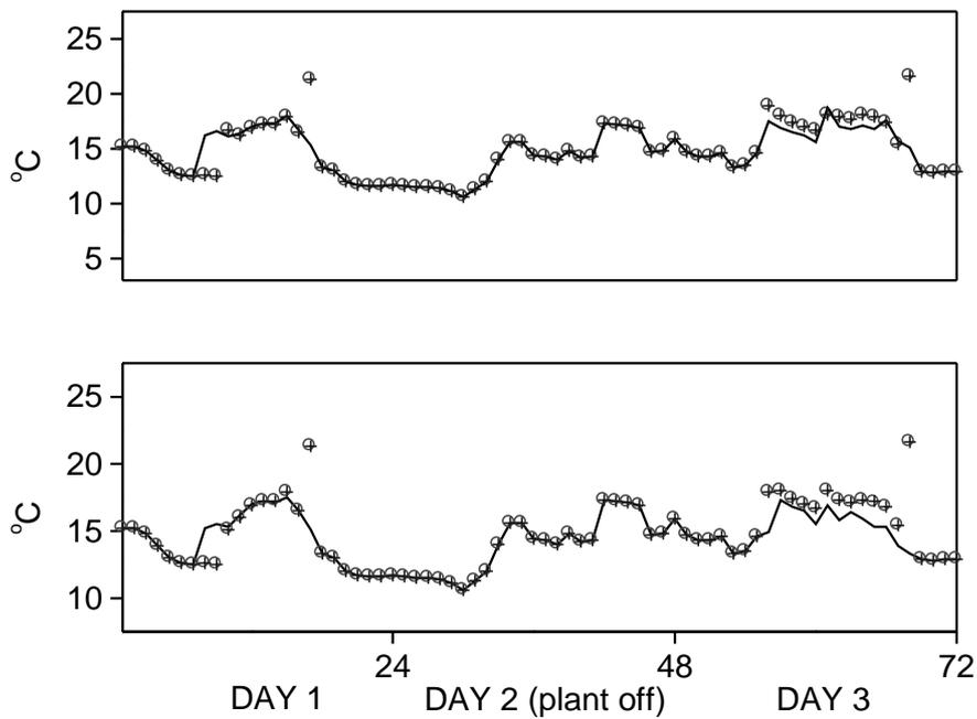
**Figure 8: summer zone supply temperatures (top: south zone, bottom: north zone)**
