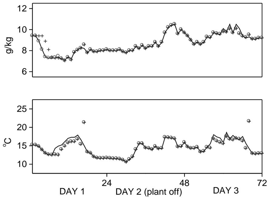
**Figure 10: summer primary air conditions (top: moisture content, bottom: temperature)**
