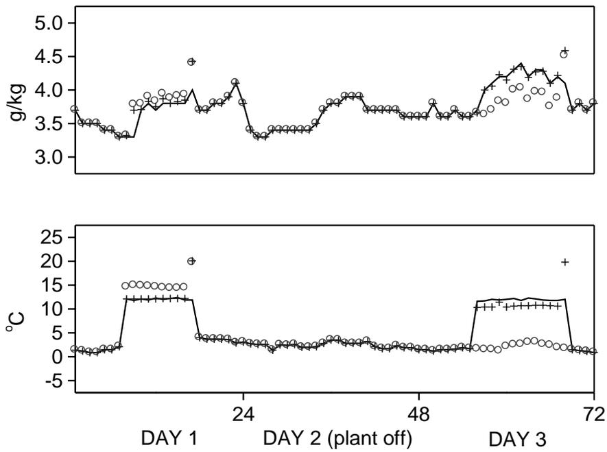
**FIGURE 9: winter primary air conditions (top: moisture content, bottom: temperature)**
