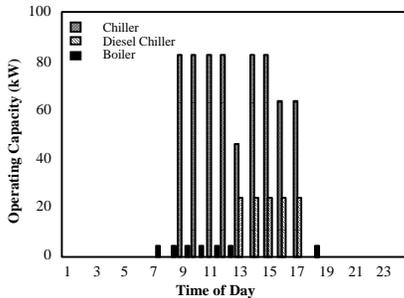
Figure 6: Minimum Cost Plant Operating Schedule for a Combination of Electric and Diesel Chillers and an Electric Boiler (Diesel Cost = 1.5/kWh)
