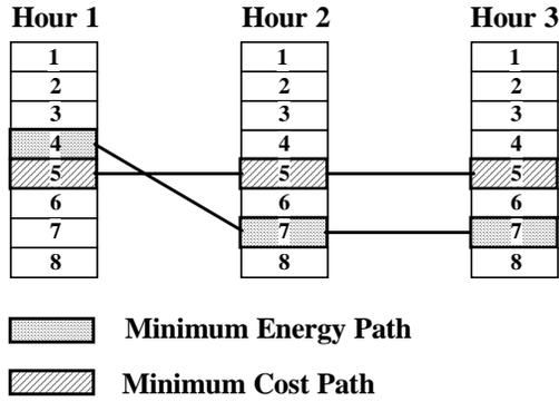
Figure 4: Determine Minimum Cost Path by Comparing Feasible Paths to Minimum Energy Path
