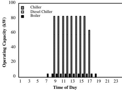
Figure 5: Minimum "Energy" Plant Operating Schedule for a Combination of Electric and Diesel Chillers and an Electric Boiler (Diesel Cost = 1.5/kWh)
