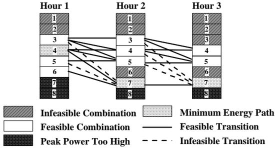
Figure 3: Determine Feasible Paths to Search by Eliminating Combinations and Transitions
