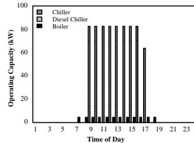
Figure 9: Minimum "Energy" Plant Operating Schedule for a Combination of Electric and Diesel Chillers and a Fuel Fired Boiler (Diesel Cost = 2.0/kWh)
