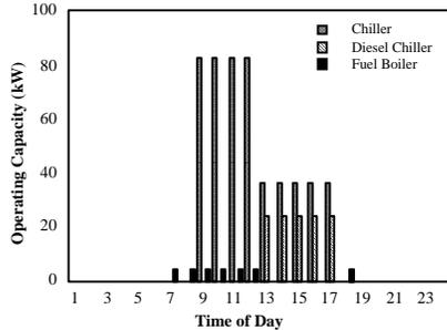
Figure 10: Minimum Cost Plant Operating Schedule for a Combination of Electric and Diesel Chillers and a Fuel Fired Boiler (Diesel Cost = 2.0/kWh)
