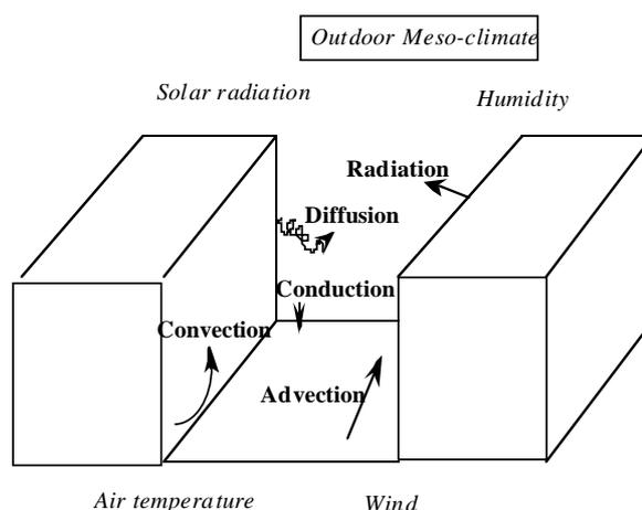
Fig 1. Overall external solicitations and internal heat flows considered in the evaluation of the urban canyon thermal answer.
