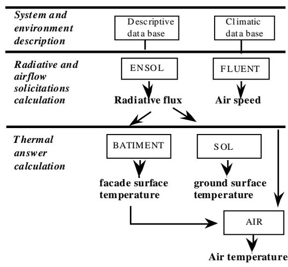
Fig 2. General layout of the Codyflow calculation code.
