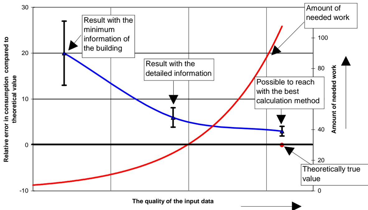
Figure 2. Relative importance of input values / different assumptions and calculation method when the target values for heating energy consumption are determined in three hypothetical cases.
