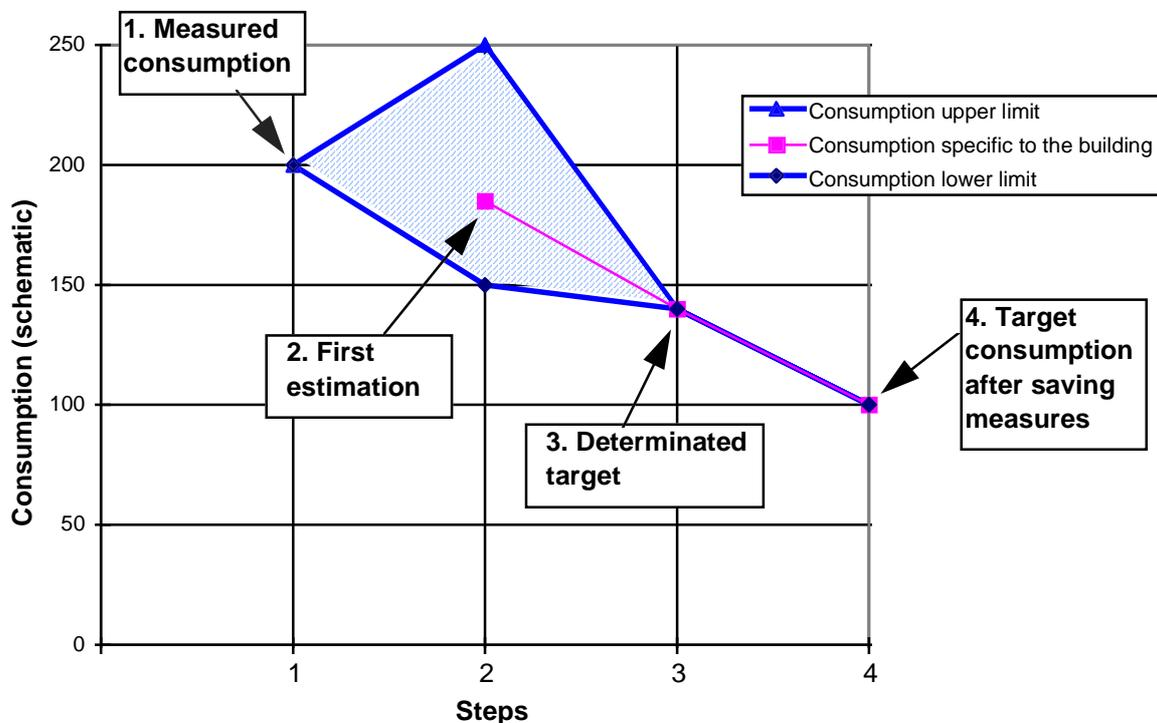
Figure 1. The calculation steps and process of energy analysis. (1) measured consumption, (2) first estimation of target consumption (3) determined target for energy consumption (4) target consumption after energy saving measures.
