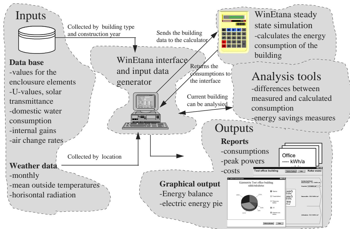
Figure 3. Different parts of the WinEtana calculation environment.
