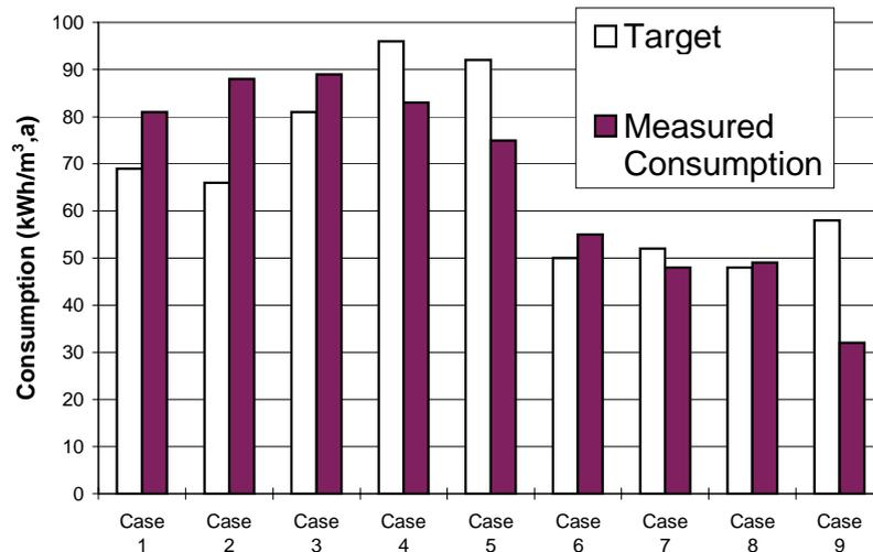
Figure 5. The calculated target and measured space heating consumptions of nine test cases.
