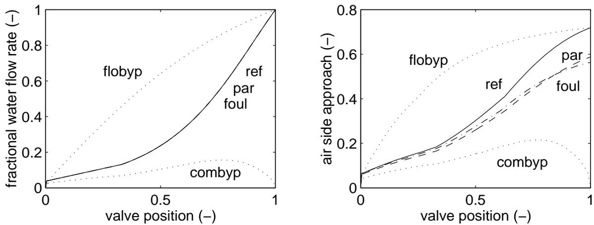
Figure 2: Cooling coil normalised water flow rates and air side approaches for correct operation ('ref'), parallel flow ('par'), fouled ('foul'), swapped flow and by-pass ports ('flobyp') and swapped common and by-pass ports ('comby')
