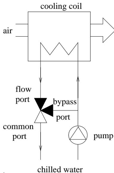
Figure 1: Cooling coil and three port control valve
