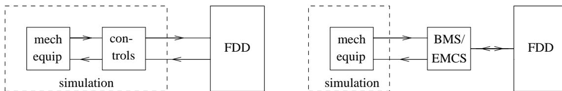
Figure 3: Methods of testing FDD procedures, left: simulated HVAC system connected to a FDD process via Unix sockets, right: simulated mechanical equipment connected to a real control system, and FDD system, via a hardware interface
