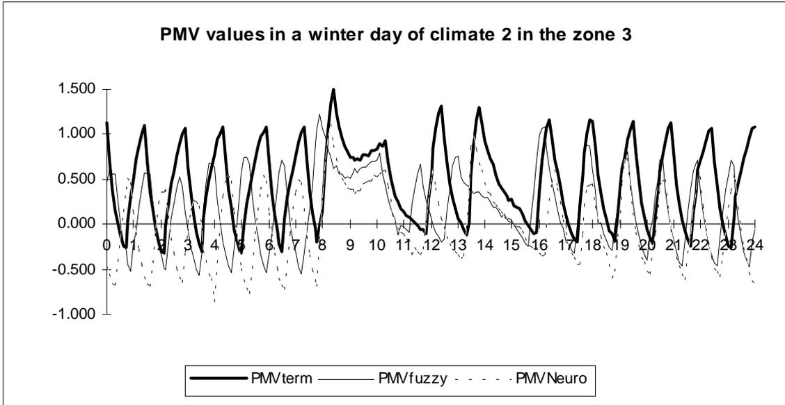
**Fig 6.** Instantaneous values of the PMV index for a simulated winter day of zone 3 in climate 2 with different controls: thermostatic, fuzzy and neuro-fuzzy.
