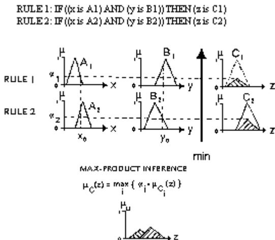
**Fig 5.** Graphical representation of the inference method used: “max-product” inference.
