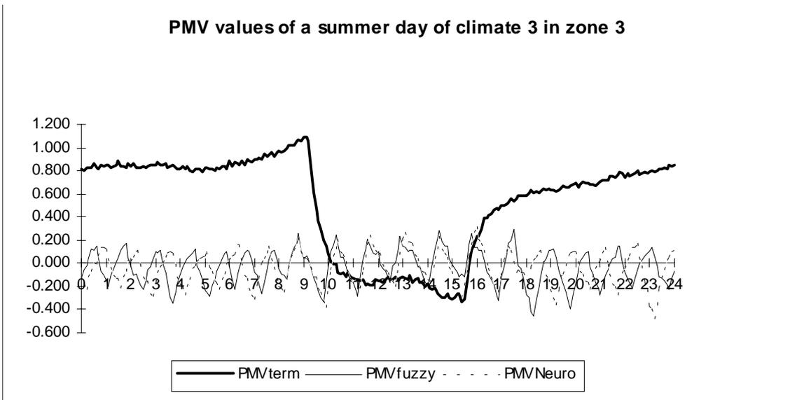
**Fig 7.** Instantaneous values of the PMV index for a simulated summer day of zone 3 in climate 3 with different controls: thermostatic, fuzzy and neuro-fuzzy.
