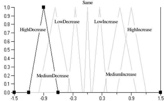
Fig 4. Adjectives of the consequent. It is the variation of fan-coils air flow rate (called “FzAirInt”).
