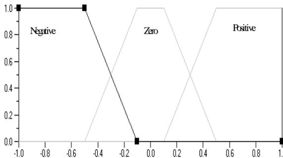
Fig 3. “FzIncFng” antecedent adjectives (represents the PMV increment from one simulation time step to the next).
