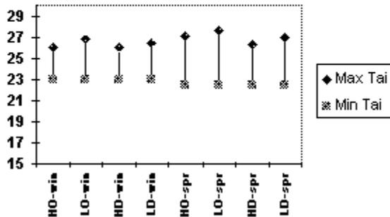
From comparison of the air temperatures in the reference zone with the air temperatures in the warmest zone (i.e. B-east 1) it follows that the temperatures in the latter zone are always about 2 C higher. This shift is due to incorrect sizing of the radiator in that room, and could easily be remedied by installation of a simple valve.
