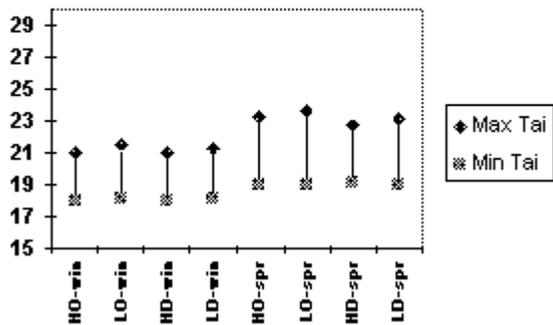
The air temperatures in the coldest zone (A-west 2), show a down-ward shift relative to the reference zone. This is due to a too small radiator in that room, which can only be remedied by changing the radiator or adding a radiator.
