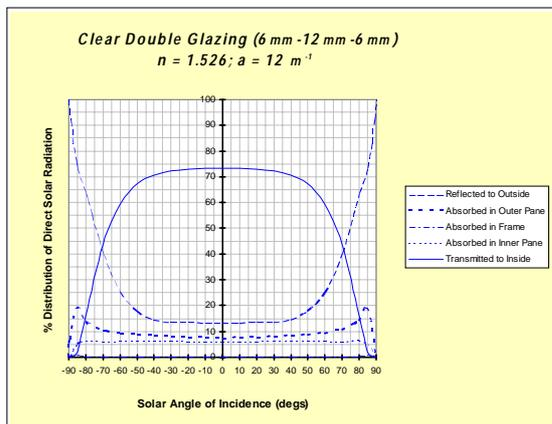
Figure 6 : Simulated Performance of Double-Glazed Window
