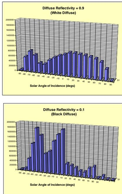
Figure 10 : The Number of Rays emitted in order to achieve Convergence for Slats tilted at +45°
