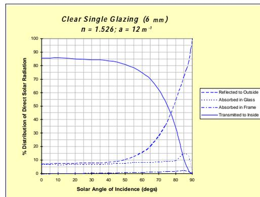
Figure 5 : Simulated Performance of Single-Glazed Window
