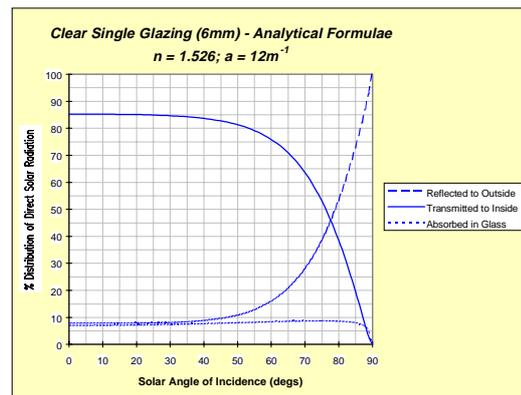
Figure 4 : Single-Glazing : Analytical Performance Curves
