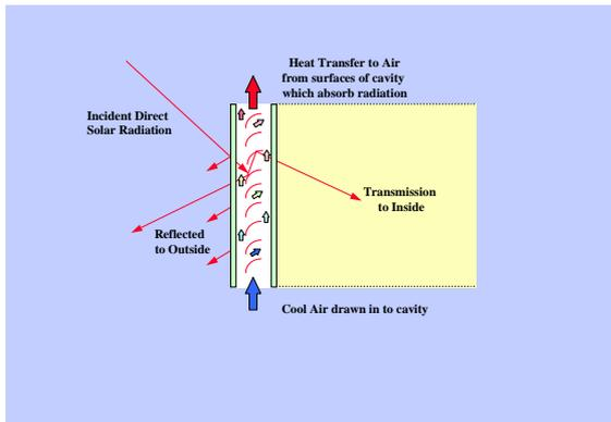
Figure 1 : Principles of Solar-induced Ventilation in a Facade containing Venetian Blinds
