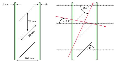
Figure 7 : Cross-Sectional Geometry for Interstitial Blinds
