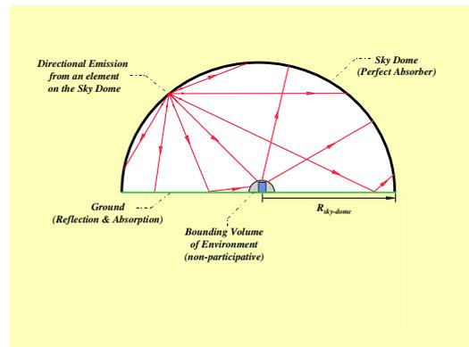
Figure 2 : Concept of Artificial Sky for simulating Diffuse Solar Radiation via 'Brute-Force' Sampling
