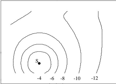
Figure 11 - Sound distribution in the test room (case 3) as predicted by CASCADE
