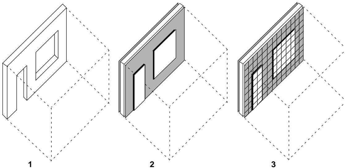
Figure 3 - Demonstrative illustration of the derivation of the CASCADE's acoustically relevant building representation from the general architectural representation in SEMPER (1: representation of an enclosure element in SEMPER; 2: CASCADE's "enrichment" of the enclosure element with acoustically relevant surface layers; 3: Segmentation of surface layers in grid elements for numeric computation purposes in CASCADE)
