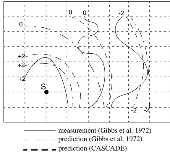
Figure 7 - Predicted and measured relative sound pressure level iso-lines
