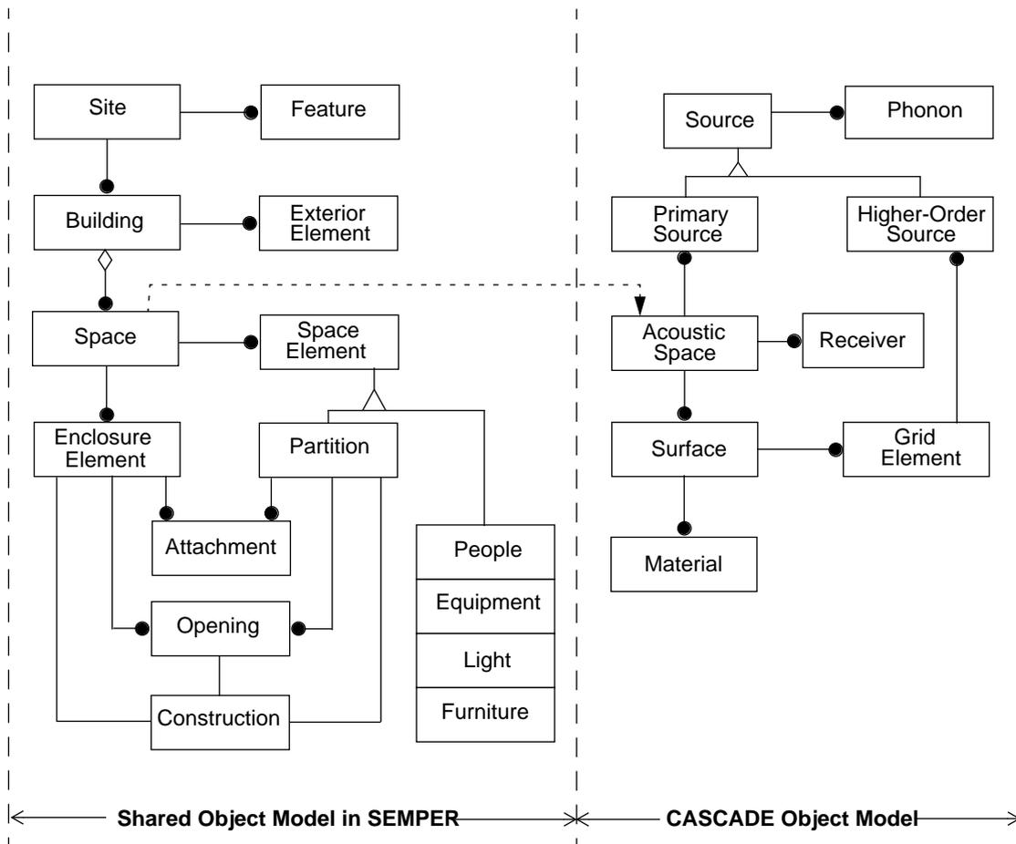
Figure 2 - SEMPER's shared object model and CASCADE's domain object model
