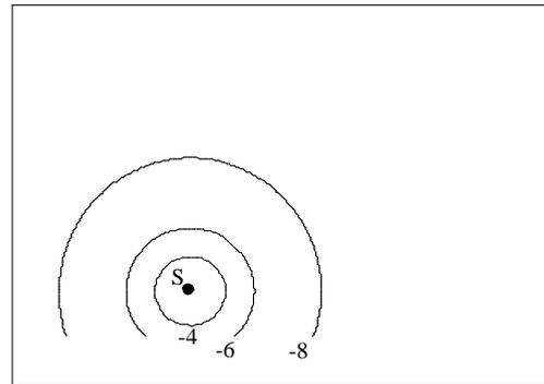
Figure 8 - Sound distribution in the test room (case 1) as predicted by the simplified method
