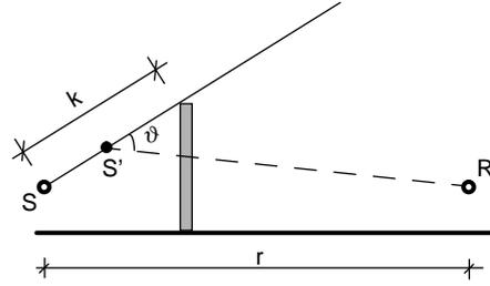
Figure 6 - Illustration of the geometric factors in diffraction modeling ( $S'$  is a reference point half-way between  $S$  and obstacle's highest point)
