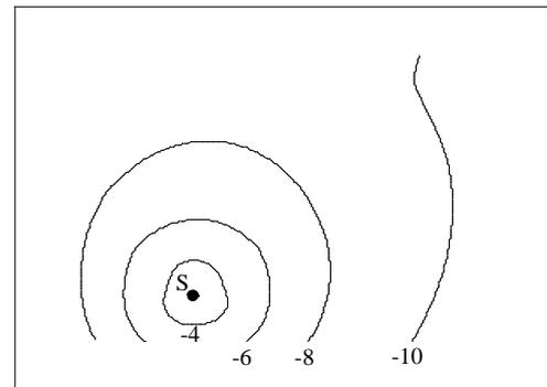
Figure 9 - Sound distribution in the test room (case 1) as predicted by CASCADE
