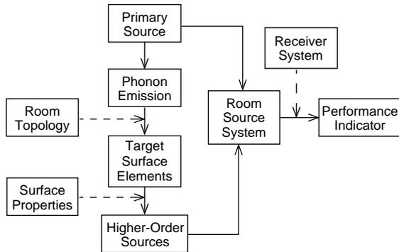
Figure 4 - Schematic illustration of the computational process in CASCADE
