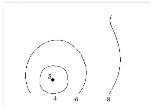
Figure 10 - Sound distribution in the test room (case 2) as predicted by CASCADE
