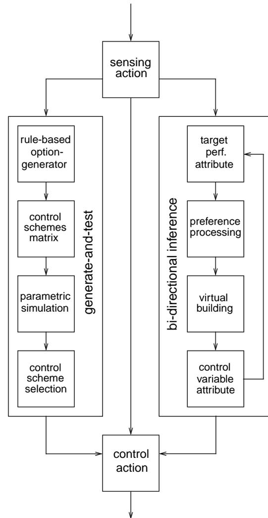
Figure 1. Schematic illustration of the use BDI and GAT for simulation-assisted building control
