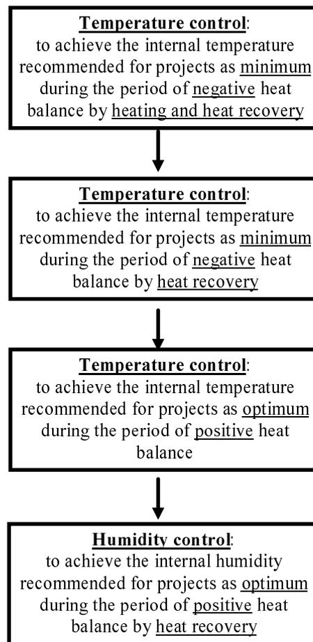
Figure 7 The purpose of use of heating and heat recovery system in different levels of ventilation
