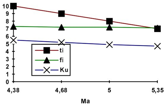
Figure 4 The program VENTOLA working screen (transformed from the VENTOLA) showing the influence of  $M_a$  on the inside air conditions ( $t_i$ ,  $\phi_i$ ,  $K_{ui}$ ) in a cowshed with negative heat balance for  $t_{ev} = -15^\circ\text{C}$
