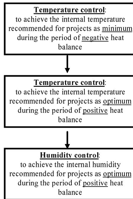
Figure 6 The purpose of use of heat recovery system in different levels of ventilation
