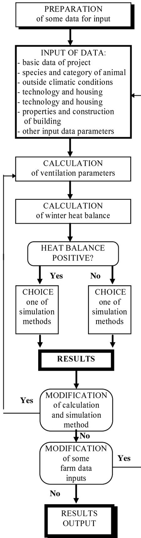
Figure 2 Overview of the model VENTOLA and its component layout
