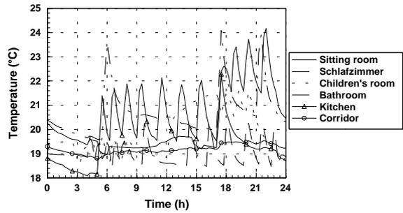
Figure 7 : Daily range of air temperature, apartment A20, single pipe heating with WRE
