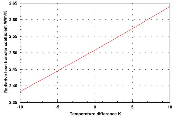
Figure 11: Radiant heat transfer coefficient in dependence on the temperature difference of two surfaces
