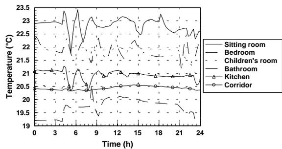
Figure 8 : Daily range of air temperature, apartment A20, single pipe heating with thermostat
