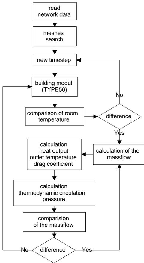
Figure 5: programming flowchart for the the heating system TRNSYS-TYPE57
