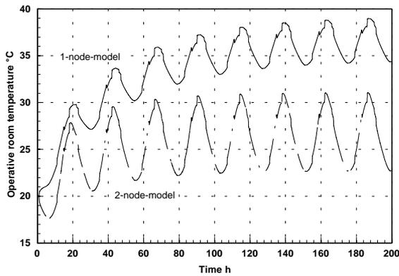
Figure 13: Oscillation of operating room temperature due to a different longwave radiation model is shown in figure 13.
