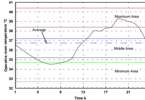
Figure 12: Operative room temperature calculated with 1-node-model
