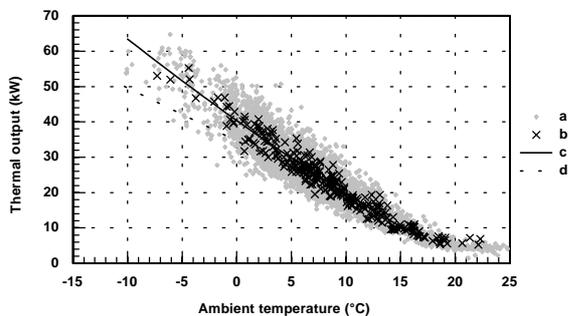
Figure 9: Average thermal output of single pipe heating as function of ambient temperature
