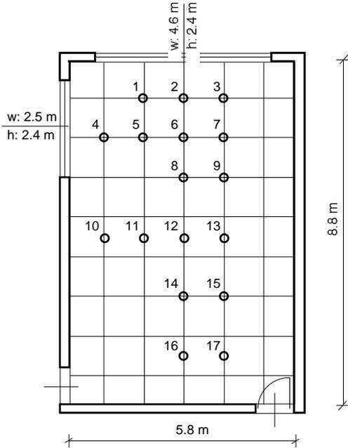
Figure 1: Schematic illustration of the test space and the location of the 17 reference points.
