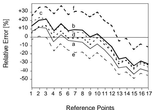
Figure 4: The relative errors of the six sky models in predicting the daylight factors for the 17 reference points in the test room. (a: CIE, b: Perez, c: Kittler, d: Brunger, e: ASRC-CIE, f: Perraudeau).
