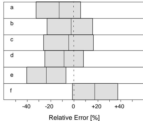
Figure 5: Mean Relative Errors with the Corresponding Standard Deviations. (a: CIE, b: Perez, c: Kittler, d: Brunger, e: ASRC-CIE, f: Perraudeau)
