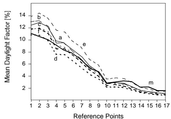
Figure 2: Mean simulated daylight factors for 17 reference points in a test room (cp. Figure 1) using six different sky models (a: CIE, b: Perez, c: Kittler, d: Brunger, e: ASRC-CIE, f: Perraudeau, m: Measured).
