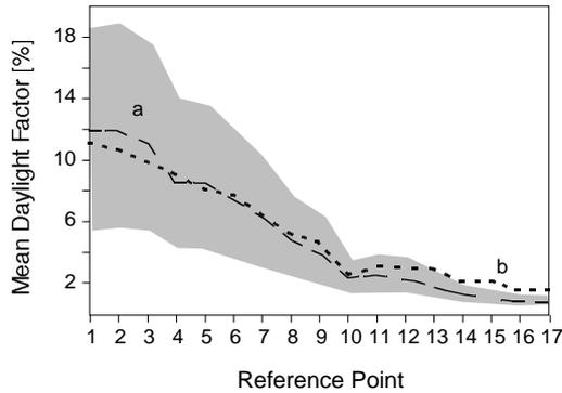
Figure 3: The predicted daylight factors (curve a) averaged over the six sky models with the corresponding standard deviations (the shaded zone). Also given is the measured average (curve b).
