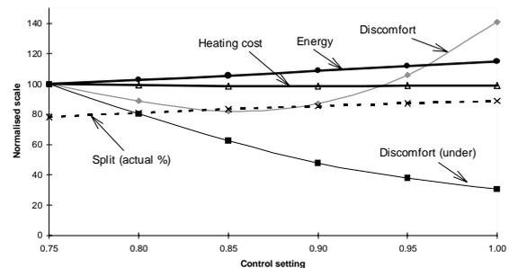
Figure 5: Variation in comfort, energy, heating cost and storage/total split as a function of control setting for manual heaters in a brick terraced house.
