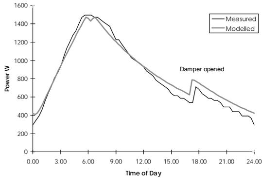
Figure 3: Graph of measured and modelled heat output from storage heater.
