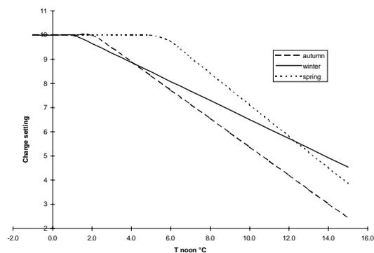
Figure 2: Control setting (1-10) against outside temperature for manual control.
