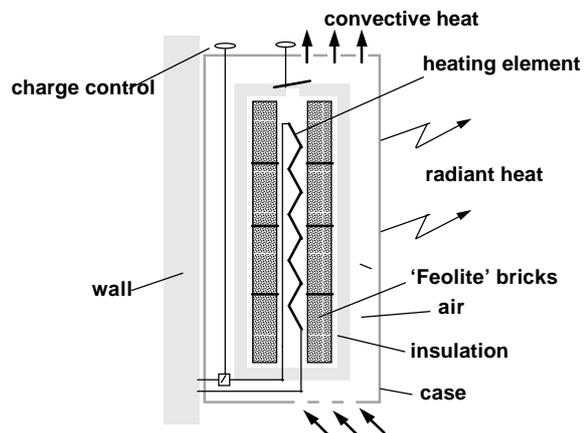
Figure 1: Cross-section of storage heater.
