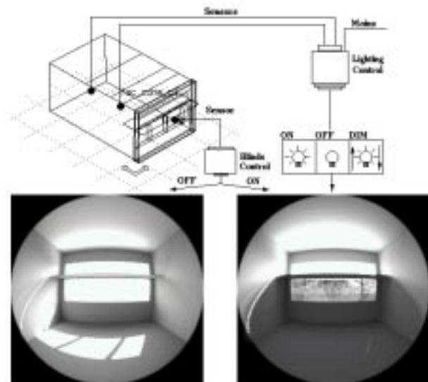
**Figure 2.** Thermal and lighting model configuration used in the lighting control case study.
