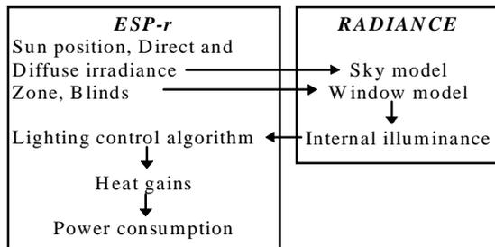
**Figure 1.** Information flows between thermal and lighting simulations at the time step level.
