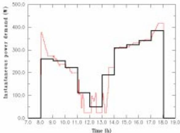
**Figure 3.** Comparison of 60 minutes (thick line) versus 5 minute (thin line) predictions of average instantaneous lighting power demand for dimming control.
