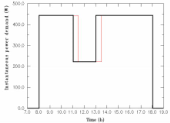
**Figure 4.** Comparison of 60 minutes (thick line) versus 5 minute (thin line) predictions of the average instantaneous lighting power demand for on - off control.
