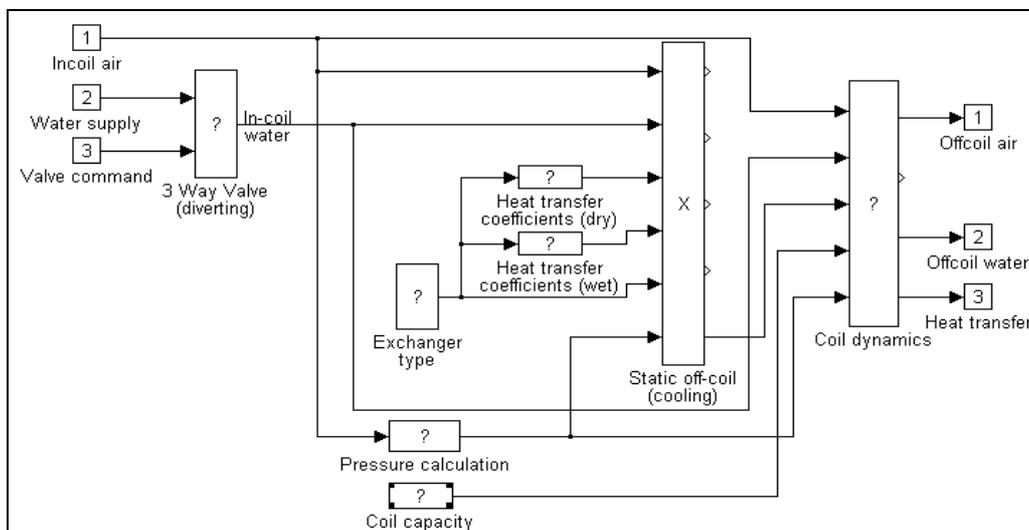
Figure 5 Simple dynamic cooling coil
