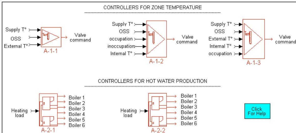
Figure 8 Controllers for hydronic heating systems
