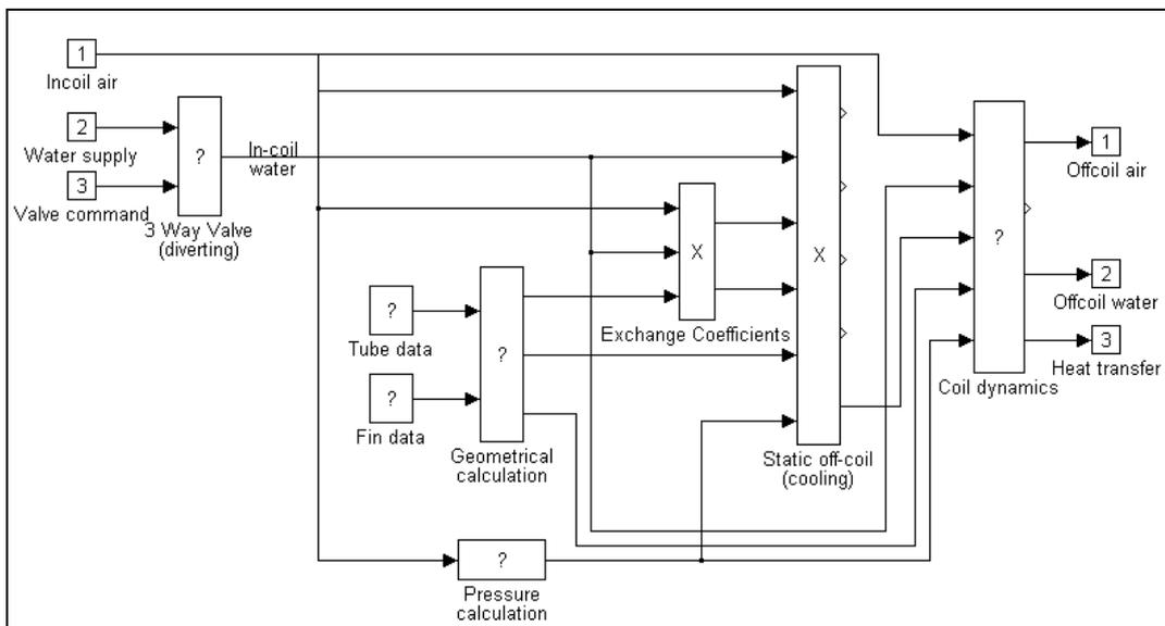
Figure 4 Detailed dynamic cooling coil
