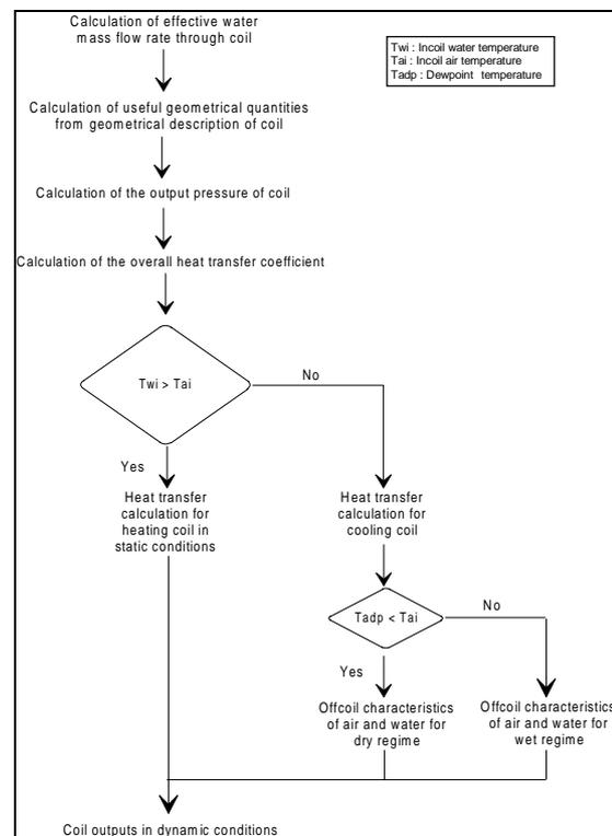
Figure 3 Flow diagram of heating/cooling coil model
