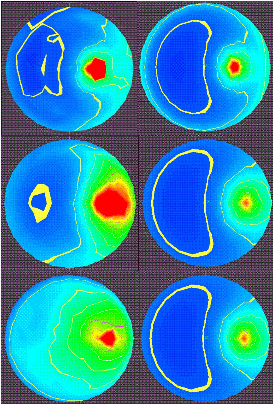
Fig. 1: Comparison of measured and simulated sky distributions according to the Perez model. Top: clear sky, middle: intermediate sky, bottom: overcast sky
