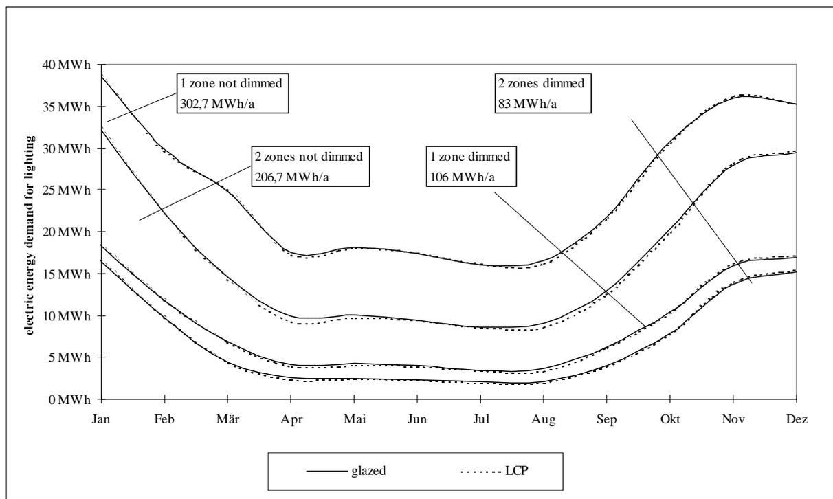
Fig. 8.: Influence of the dimming of light on the electrical energy demand for light. Two design options are considered: Glazing and Laser Cut Panels (LCP).
