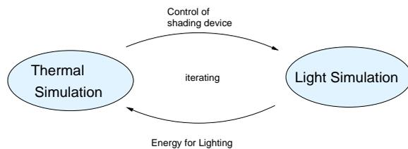
Fig. 4: Schematic view of the interaction between the light and the thermal calculations
