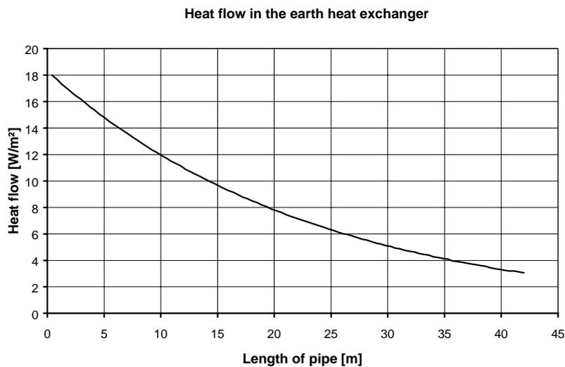
Figure 3: Heat flow along the pipe of the earth heat exchanger for a winter day (calculated by *GAEA*)
