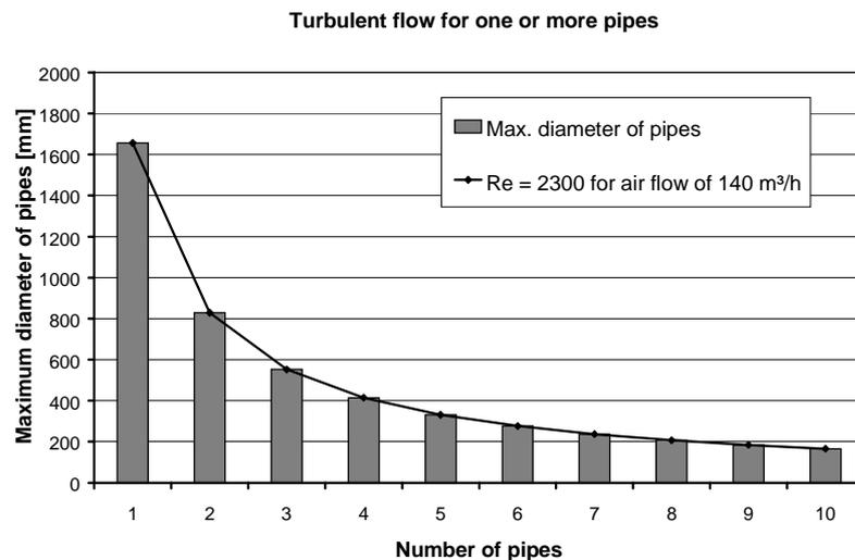
Figure 6: Conditions for turbulent flow in earth heat exchangers with one or more pipes
