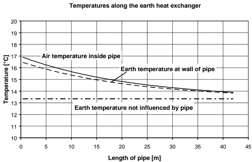
Figure 2: Temperatures along the pipe of the earth heat exchanger for a warm summer day (calculated by *GAEA*)
