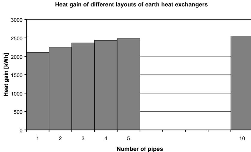
Figure 7: Comparison of different earth heat exchanger layouts
