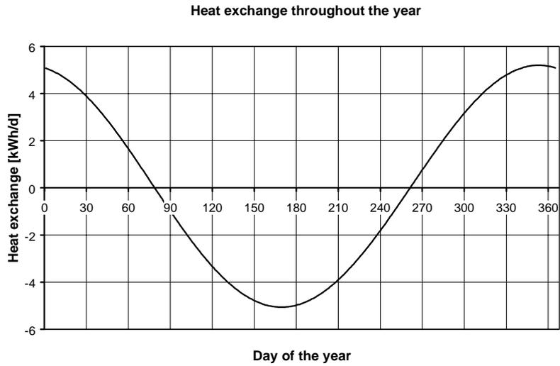
Figure 4: Heat exchange in the earth heat exchanger throughout the year (calculated by *GAEA*)
