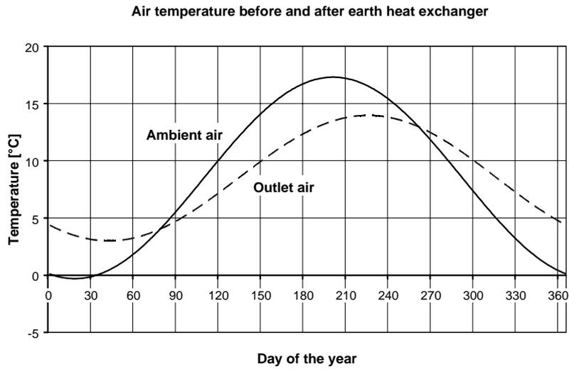
Figure 1: Ambient air temperature and temperature at the outlet of the earth heat exchanger throughout the year (calculated by *GAEA*)
