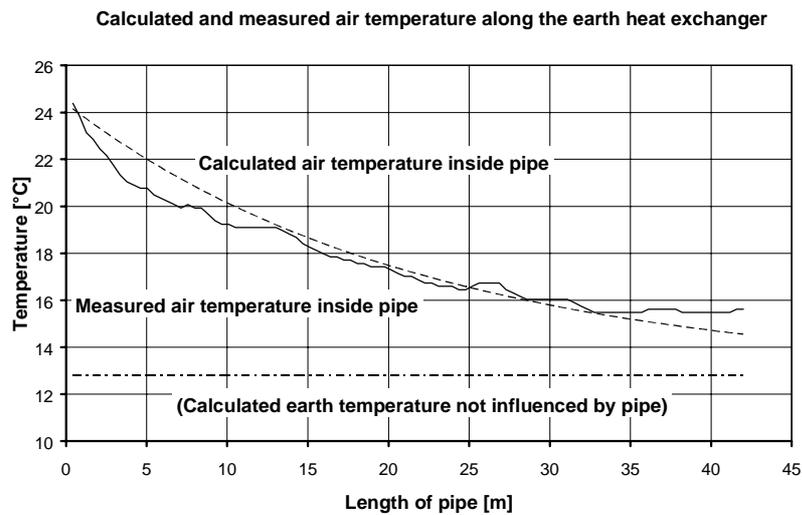
Figure 5: Comparison of measured and calculated air temperatures for a warm summer day along the earth heat exchanger
