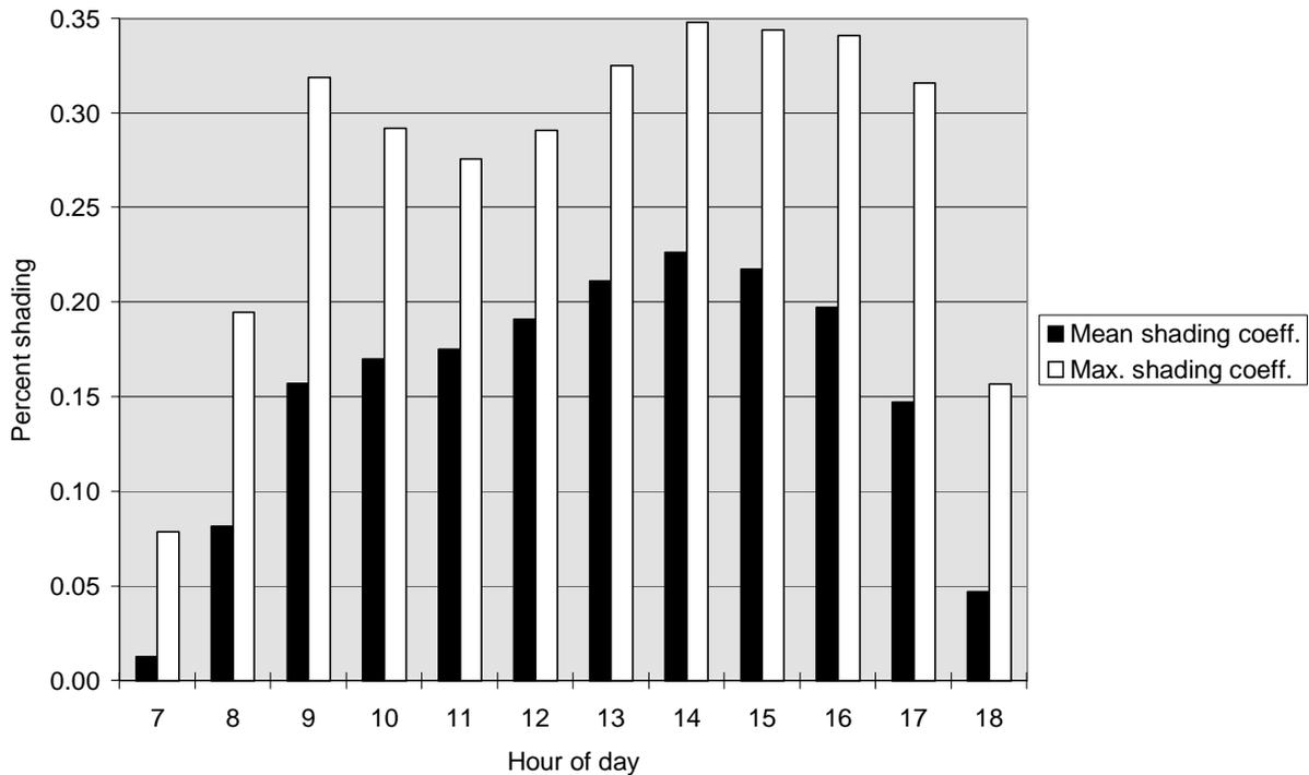
Figure 8: Mean and maximum values of shading of the south façade for the whole year.
