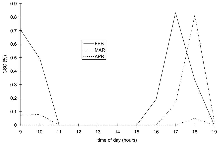
Figure 5: GSC as a function of time of day for the months of February to April. The shaded target is an area of 2 m height times 4 m width in the upper left corner of the roof. The diagram is similar to SOMBRERO's online output window.
