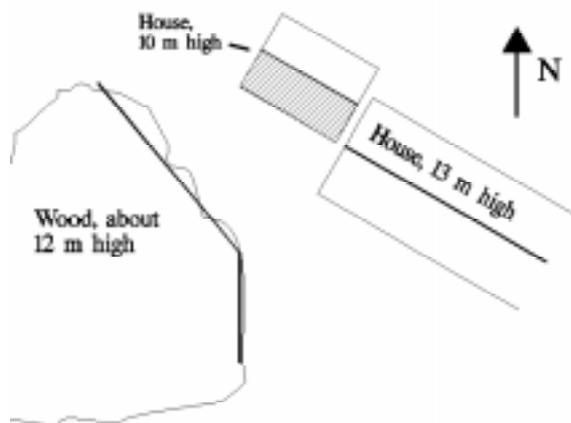
Figure 3: Ground plan of the building on which the collector shall be mounted and of the shading elements.
