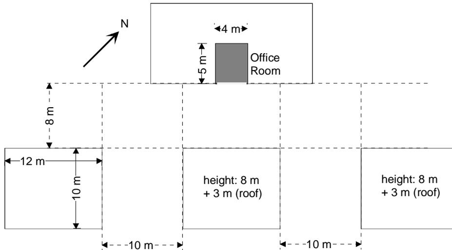
Figure 1: Site plan of the office room. Window orientation is south-east, the size of the window is 3.5 m x 2 m, the window-sill is situated 3 m above the ground.
