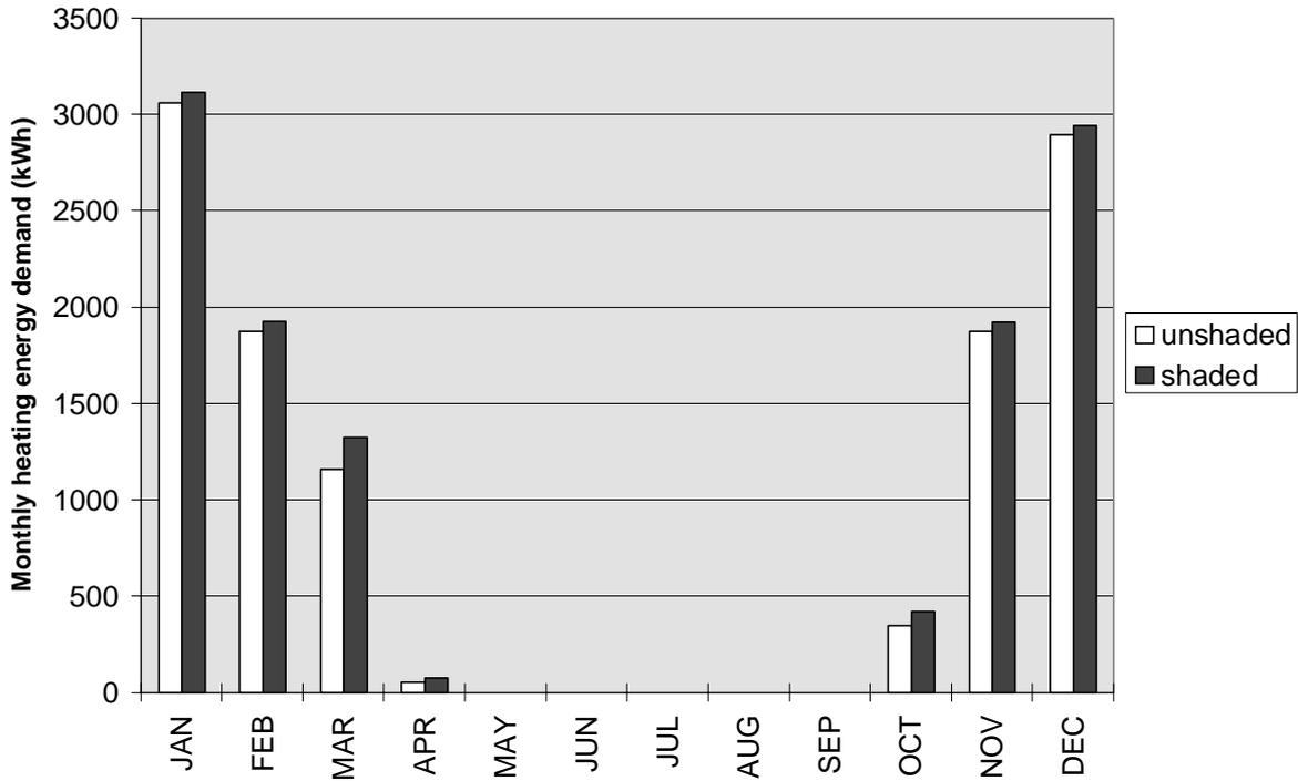
Figure 7: Total monthly heating energy demand for the building with and without the shading trees.
