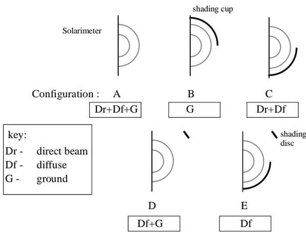
Figure 3 - Solarimeter cell masking configurations
