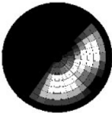
Figure 5 Example visualisation of an HTB2 shading mask, containing overhang, sidefin, and site obstructions.
