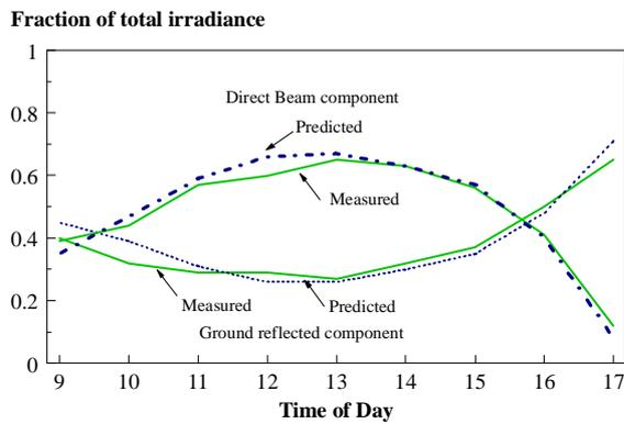
Figure 11 Comparison of measurement and prediction of the solar components for the vertical side-fin shaded case.
