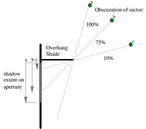
Figure 4 Principles of an HTB2 shading mask
