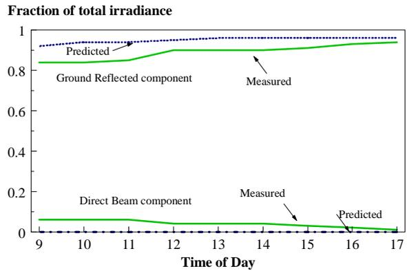
Figure 12 Comparison of measurement and prediction of the solar components for the "egg-crate" shaded case.
