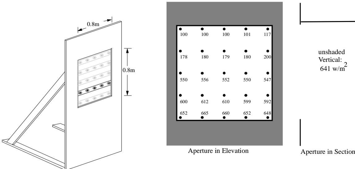
Figure 1 - Sketch of test window aperture and measurement rig, showing scanning
