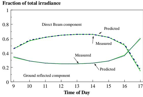
Figure 9 Comparison of measurement and prediction of the solar components for the unshaded case.
