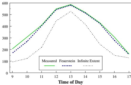
Figure 7 Comparison of measurement and prediction of total solar irradiance for the vertical side-fin shaded case.
