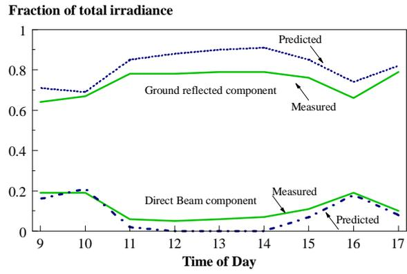
Figure 10 Comparison of measurement and prediction of the solar components for the horizontal overhang shaded case.
