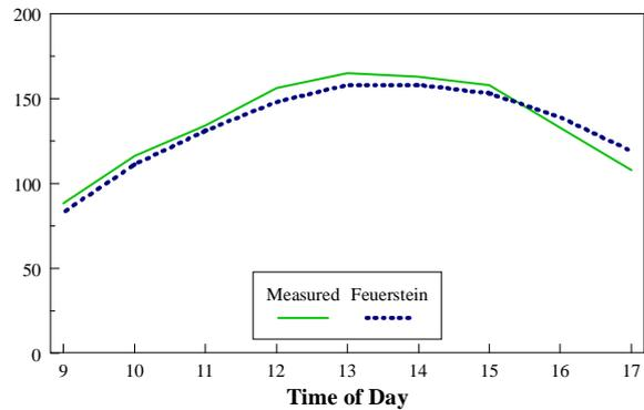
Figure 8 Comparison of measurement and prediction of total solar irradiance for the "egg-crate" shaded case.
