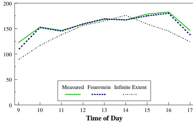
Figure 6 - Comparison of measurement and prediction of total solar irradiance for the horizontal overhang shaded case.
