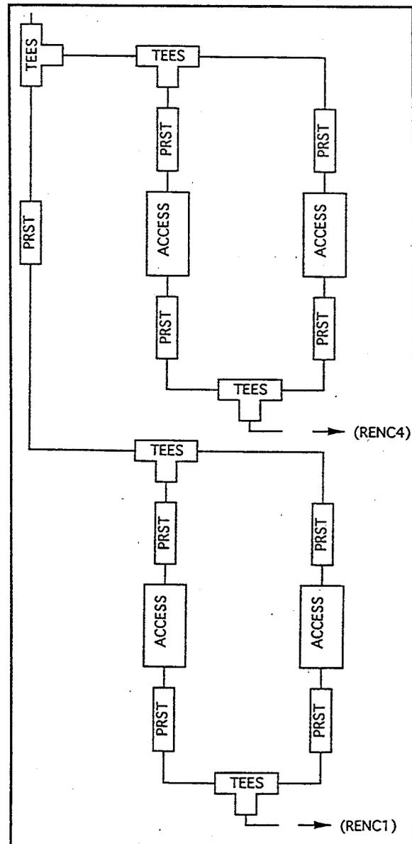
Figure 2. Supply A, Non-Hazardous Ventilation System SAN
