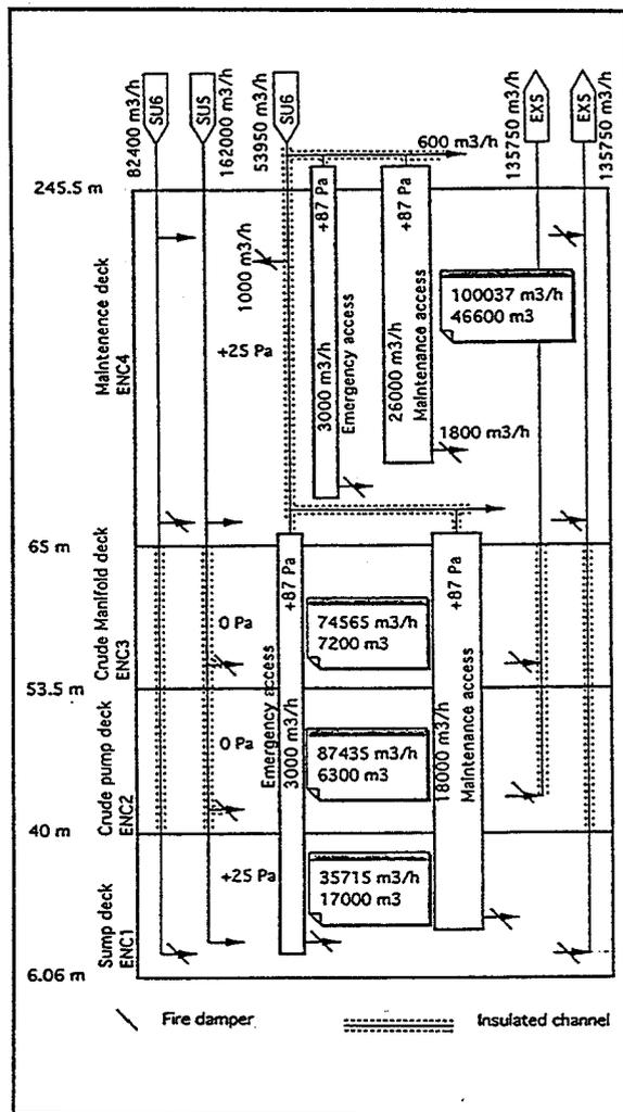
Figure 1. Schematic Description of the Ventilation System
