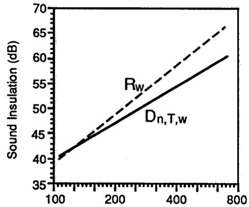
Fig. 5 Deviation of the effective sound level difference between two adjacent rooms in a typical massive construction from the sound reduction index of the partition element as a function of the surface density of the partition element.
