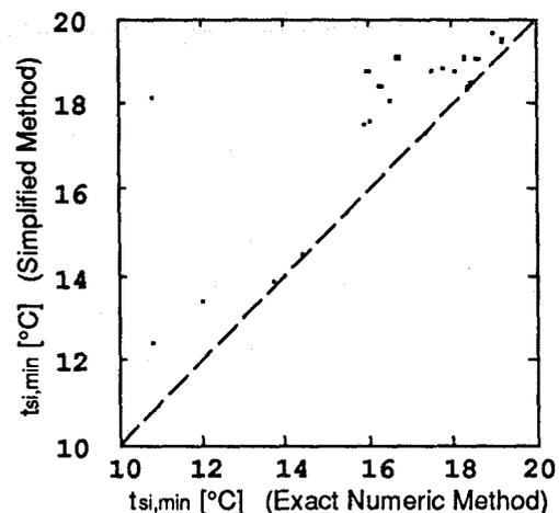
Fig. 2 Comparative analysis of indoor surface temperatures for 30 residential constructions using different simulation methods.
