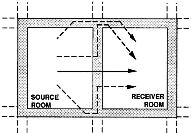
Fig. 3 Direct and Flanking Sound Propagation Paths Between Adjacent Spaces
