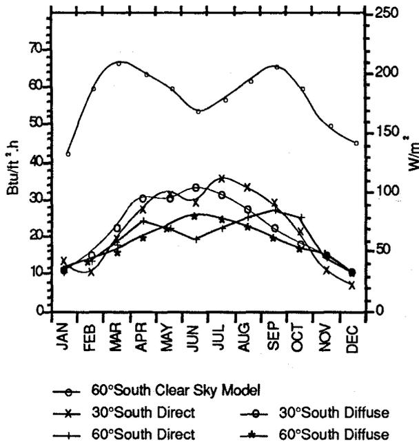
Fig. 6 Diffuse and direct components of the solar irradiance incident on south sloped surfaces (30° and 60°) based on extensive hourly simulation, compared with the result obtained by applying a simple clear sky model for direct component on a 60° pitch south facing surface.
