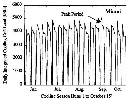
Figure 1.b: Daily Integrated Cooling Coil Loads in Miami.
