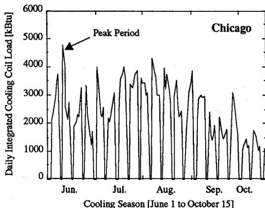
Figure 1.a: Daily Integrated Cooling Coil Loads in Chicago.
