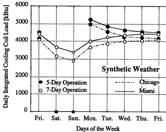
Figure 3: Daily Integrated Cooling Coil Loads for a Week of Synthetic Weather in Chicago and Miami.
