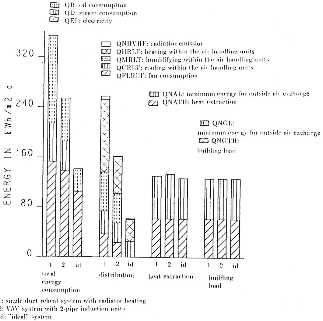
Figure 3: Comparison of the energy consumption of two air conditioning systems and an ideal system, yearly results
