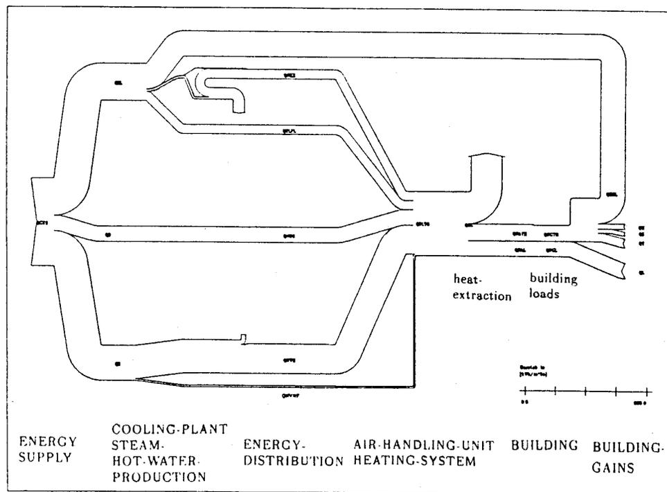
Figure 2: Energy flow diagram for an office building with single duct constant volume air conditioning system with perimeter radiator heating, yearly results
