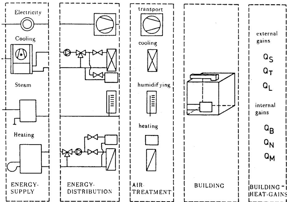
Figure 1: Important Subsystems and Boundaries within a Building and HVAC-System
