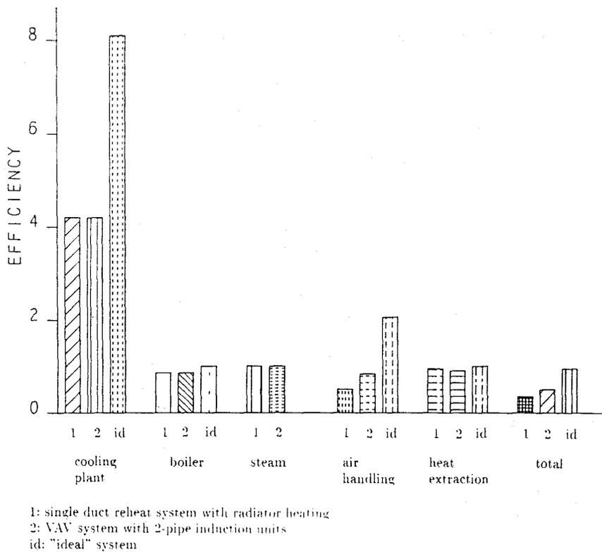
Figure 4: Comparison of the yearly efficiencies of two air conditioning systems and an ideal system
