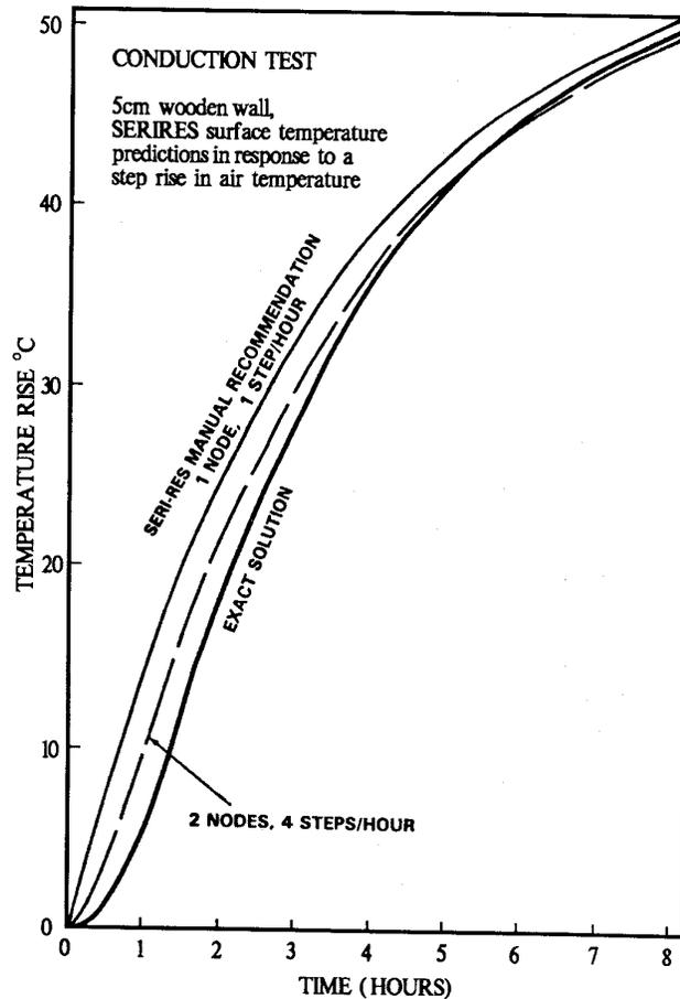
FIG. 1 Results of BRE Analytical Test for SERIRES Conduction Algorithm
